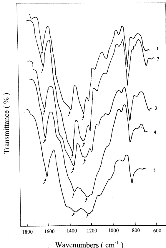
Fig. 1. Infrared spectrum of boron-containing bisphenol-A formaldehyde resin (1) uncuring, (2) 120°C, (3) 140°C, (4) 160°C, and (5) 180°C curing 1.5 h.
