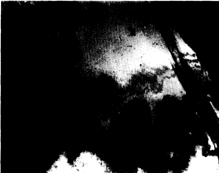
Fig. 27. Optical micrography under crossed polarizers at room temperature of a DOMS-SA film stretched at 35°C up to \lambda = 1.8 and rapidly cooled down to the glassy state. (Reproduced by permission of Hüthig & Wepf Verlag.)
