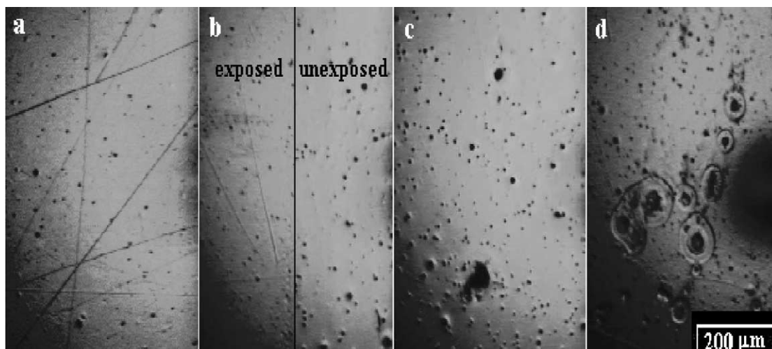
Fig. 7. Optical micrographs of vinyl ester surface after (a) 0 h, (b) 1000 h at interface between unexposed and exposed surfaces, (c) 1000 h, and (d) 4000 h of exposure.
