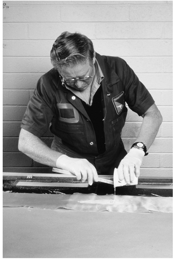
Fig. 16. If required, additional adhesive is poured onto the fibreglass and again spread with a brush or a squeegee.
