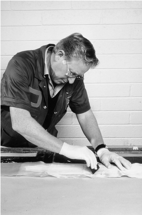
Fig. 15. The Epocast ® 50A resin and 9449 hardener are mixed thoroughly and brushed onto the clean panel surface. Dry fibreglass plies are then positioned into the wet resin and the laminating system is pulled through the cloth with the aid of a squeegee which also helps in removing trapped air beneath the cloth.
