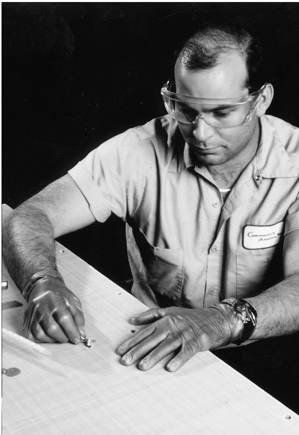
Fig. 1. Once cut to size, tabbed inserts required to attach flooring to the aircraft are bonded into the panels.
