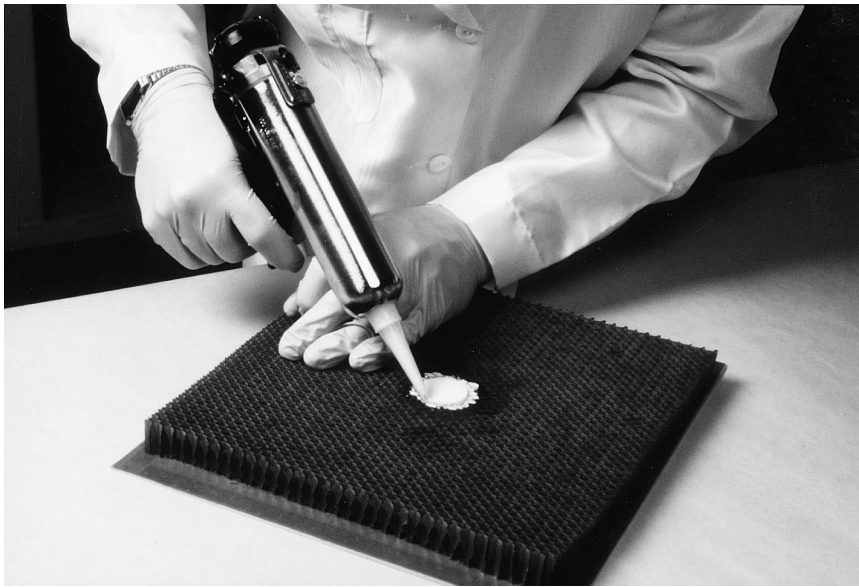
Fig. 11. Alternatively, the honeycomb core can be reinforced by applying a paste syntactic such as Ciba's Epocast ® 1614-ATF or CG 1305 around the insert until the surrounding honeycomb cavities are completely filled.
