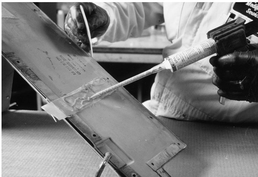
Fig. 5. For reinforcement, several more beads of adhesive are then dispensed over the top of the fibreglass.
