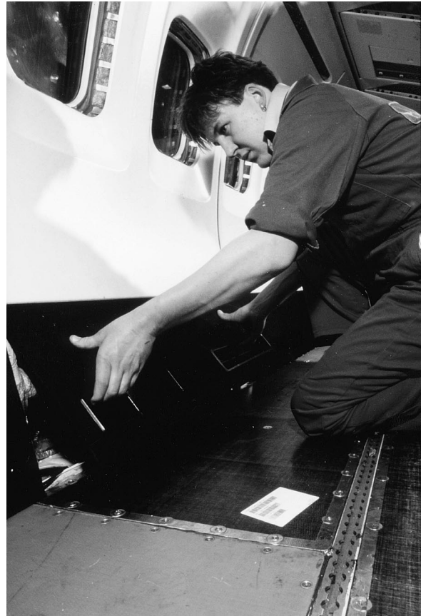
Fig. 18. After the curing cycle is complete, the panel is covered with carpet and reinstalled into the aircraft.
