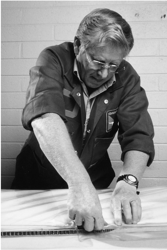
Fig. 17. When the laminate is complete, the structure is vacuum bagged using a layer of release film and a breather cloth. The part is then allowed to cure overnight.
