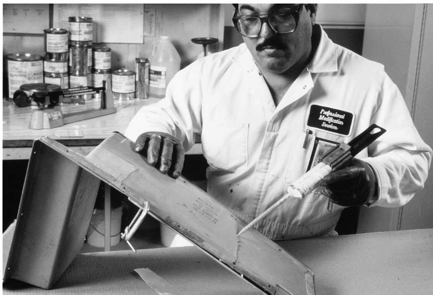
Fig. 3. A PMS technician begins by applying a bead of adhesive from an Accumix ® cartridge into the crack.
