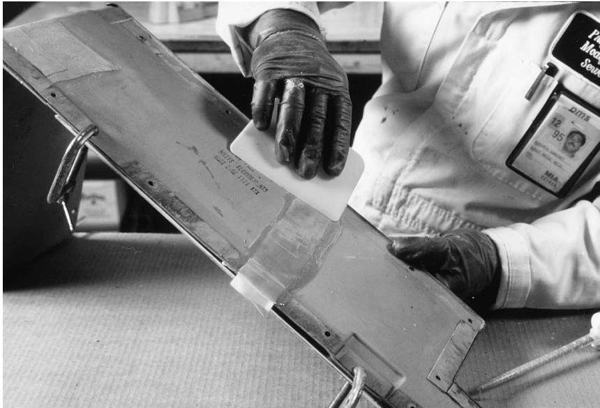
Fig. 6. Resin is spread across the cloth with a squeegee to ensure that the cloth is thoroughly wet-out.
